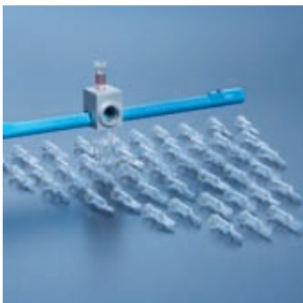
Analysis of the cell volume with the PCV packed cell volume tube and «easy read».
